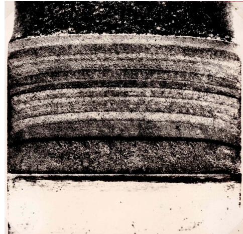
Fig. 4. Stepwise interrupted fatigue crack growth
